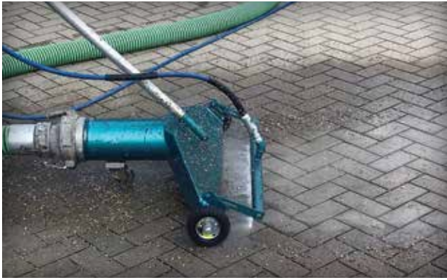
Figure 23. This equipment provides combined washing and vacuum of unmaintained PICP.
